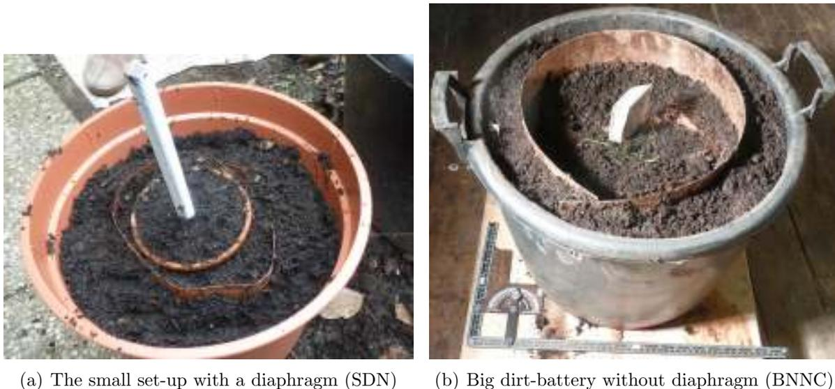
Figure 3.8.: Two different set-ups of dirt-batteries
